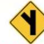
Road branching off left
